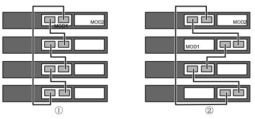
Figure 3-27 Cable connections in an IRF in the non-aggregate mode with 2-port interface modules
